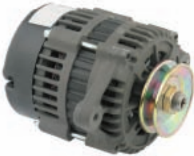
9-19109 Alternator (New) 70 amp Replaces: Mercruiser 862030T, Delco 19020616, Delco alternator 12V, 70 amp internal regulator, v-belt pulley
