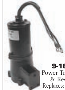
9-18600 Power Tilt Motor Replaces: OMC 982058, 982706 Fits: OMC Sterndrives 1980-85, Prestolite EVD4001 & EVD4002, 3-wire connection
