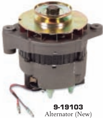
9-19100 Alternator (New) Replaces: Mercruiser 69729 Delco Alternator, 12V, 61 amp, Self-exciting regulator, 1 wire hook-up, v-belt pulley
